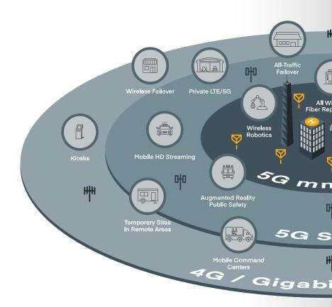
The Sub-6 band requires greater densification than 4G LTE, and therefore will be less pervasive. Since Sub-6 has significantly better performance compared to 4G LTE, high-bandwidth applications will run capably.
